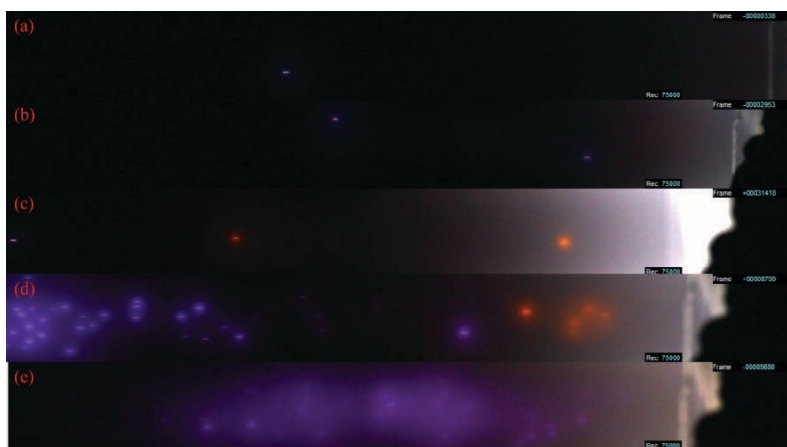
Figure 6. Experimentally captured ion cloud trajectories of different particles in the ICP tail flame: (a) \text{Er}_2\text{O}_3 , (b) \text{Y}_2\text{O}_3 , (c) BSG_10, (d) BSG_5, and (e) BSG_2.
