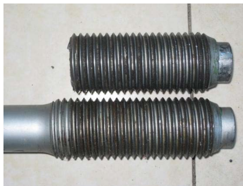
Figure 9. Comparison diagram of bolt fracture positions.
